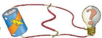
Students will need a circuit modified like the one shown in the illustration. (Strip a 1-inch section of insulation off the middle of each wire). Students will also need a 6-inch piece of thicker wire with 1 inch of insulation removed at each end.
